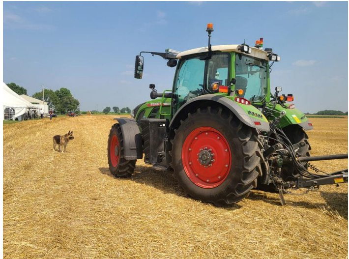
AGCO's autonomous tractor encountered a dog in its path and stopped automatically
